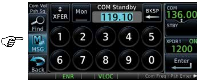
COM Standby Screen
